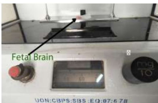
Figure 2.5: Showing how fetal brain weight was taken using a weighing scale from Oertring company-Japan model
